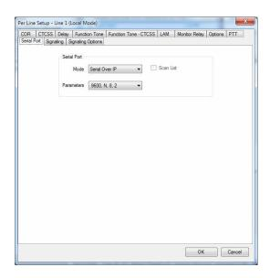
Change the Parameters value to 9600,N,8,1 by clicking the arrow and selecting from the list, as shown in the example below.
