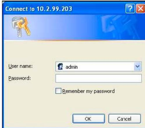
*If this is the first time the IP-223 has been started and a password has not been assigned to the unit, no entry is required.*
